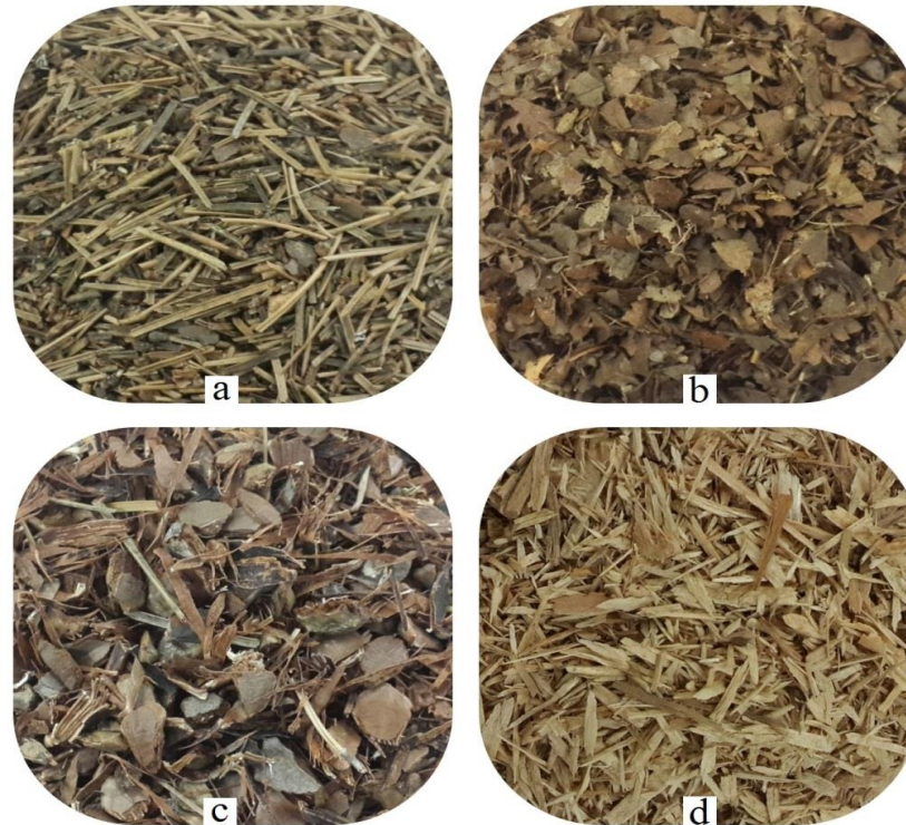
Fig. 1. The raw materials used in the production of particleboard: a) needle litter; b) broad-leaf; c) pine cones; d) WP
