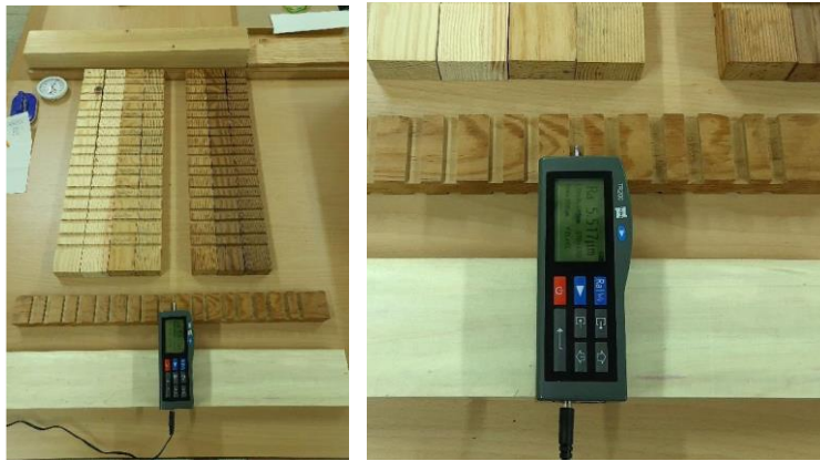
Fig. 4. Roughness measurement in wood specimens
