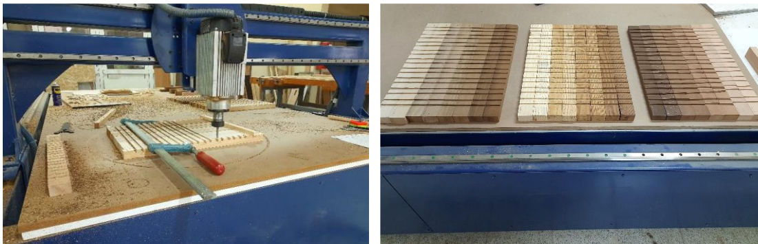
Fig. 2. Cutting specimens with CNC router machine
