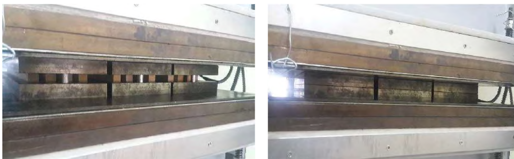
Figure 1. Densification of specimens by using metal molds
