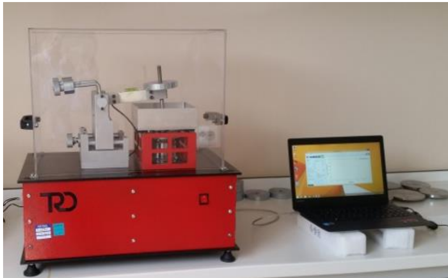
Figure 3. TRD Wear abrasion tester.
