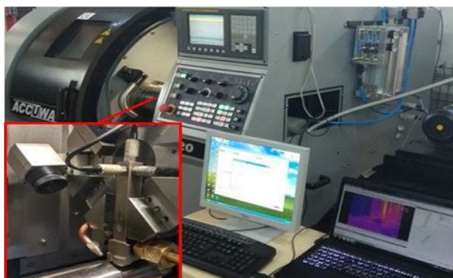
Fig. 1 – CNC lathe and MQL system experimental setup.
