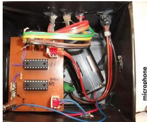
Figure 7. Microcontroller and voice detection card.
