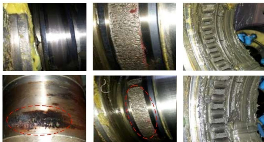
Figure 8. Common defects of inner race generator rolling bearings of wind turbines. Reproduced from [85], Elsevier.
