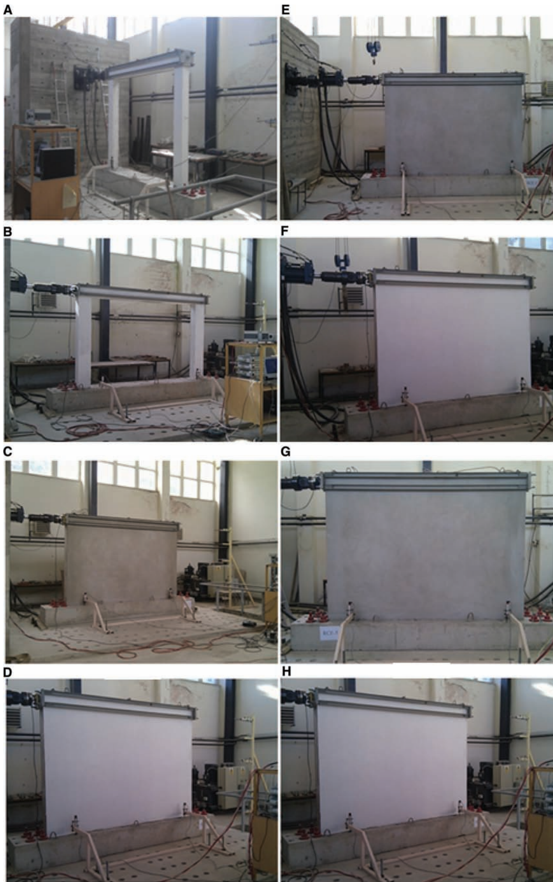
Figure 6: General views of test frames under lateral reversed cyclic loading. (A) PRCF-1, (B) PRCF-2, (C) RCF-1, (D) RCF-2, (E) RCF-3, (F) RCF-4, (G) RCF-5, (H) RCF-6.
