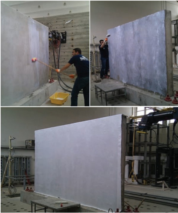
Figure 3: Application steps of glass fiber reinforced polymer sheet to the infilled reinforced concrete (RC) frames.
