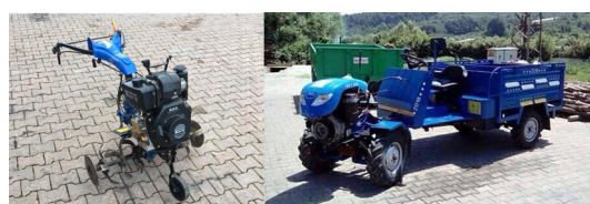
Figure 1 Agricultural machines with grubber or single-axle two-wheel tractor is called pat-pat.
