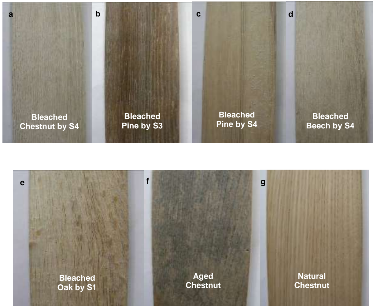
Fig. 5. (a) Chestnut sample bleached by S4, (b) Pine sample bleached by S3, (c) Pine sample bleached by S4, (d) Beech sample bleached by S4, (e) Oak sample bleached by S1, (f) Aged chestnut sample, (g) Natural chestnut sample
