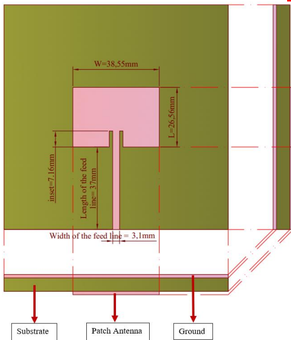
Figure 1. Dimensions of the antenna
