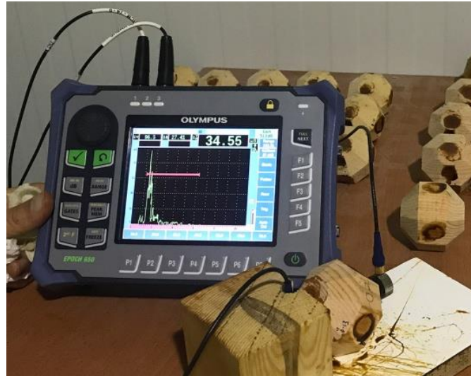
Fig. 2. Time of flight measurements of ultrasonic shear wave.
