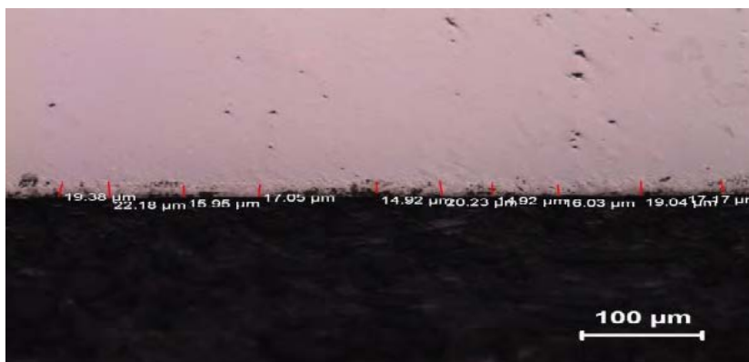
FIGURE 5. Microstructure of boron coated AISI D2 cutting tool.
