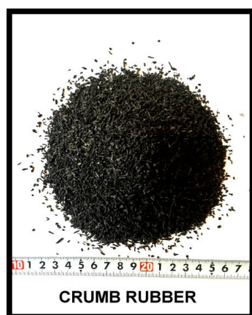
Fig. 3. Rubber granule within 1-2 mm sieve range
