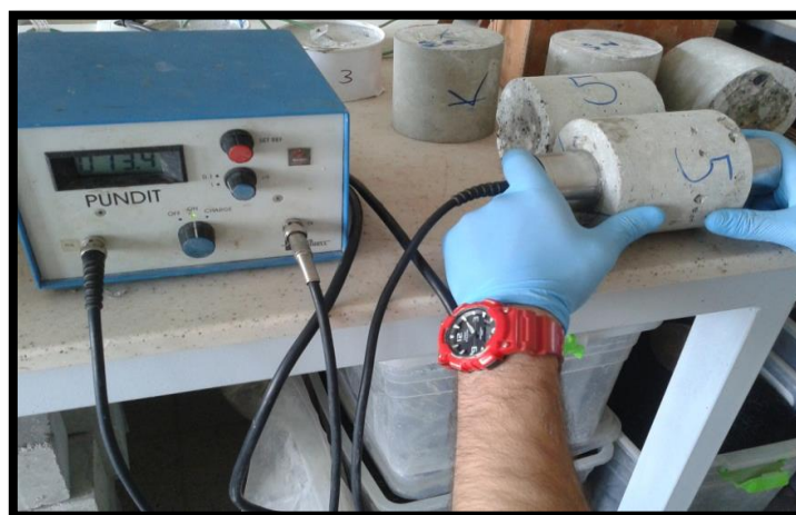
Fig. 5 Application of ultrasonic pulse velocity test
