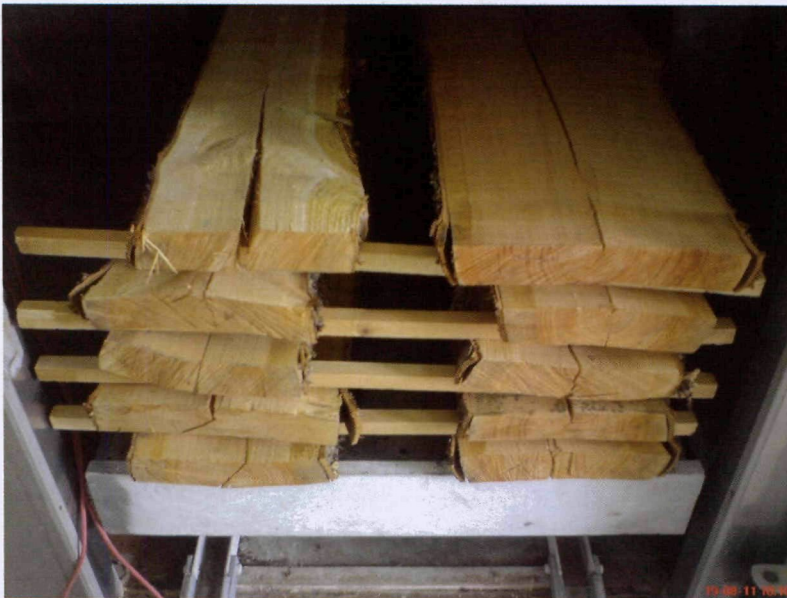
Figure 6. View of lumbars dried with non-protective drying schedule.
